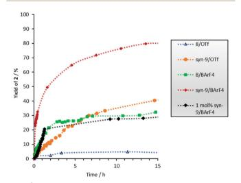
Fig. 4 <sup>1</sup>H-NMR yield vs. time profile for the formation of cyclopentenone 2. The error is approximately 5%.  $c_0(\mathbf{1}) = 15.4 \text{ mM}.$
