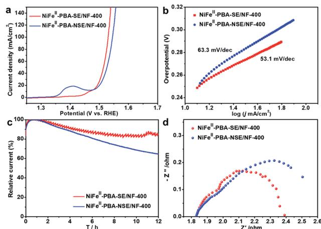
Fig. 5 (a) *iR*-corrected linear sweep voltammetry (LSV) curves, (b) corresponding Tafel plots of the catalysts with and without encapsulation, and (c) the durability measurements of NiFe<sup>II</sup>-PBA-SE/NF-400 and NiFe<sup>II</sup>-PBA-NSE/NF-400 under a constant potential of 1.6 V (vs. RHE). (d) Nyquist plots of the catalysts with and without encapsulation with a potential of 1.6 V (vs. RHE).
