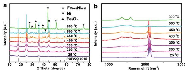
Fig. 1 (a) XRD patterns and (b) Raman spectra of the  $\text{NiFe}^{\text{II}}$ -PBA crystals after heat treatment at different temperatures ( $25^\circ\text{C}$  represents initial  $\text{NiFe}^{\text{II}}$ -PBA without heat treatment).
