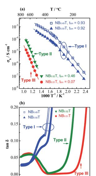
Fig. 1 (a) Arrhenius plot of bulk conductivity,  $\sigma_{\rm b}$  and (b) dielectric loss, tan  $\delta$ , at 1 MHz versus temperature for NBT with various A-site Bi nonstoichiometry:  $Na_{0.5}Bi_{0.49}TiO_{2.985}$ ,  $NB_{0.49}T$ ;  $Na_{0.5}Bi_{0.5}TiO_3$ ,  $NB_{0.50}T$ ;  $Na_{0.5}Bi_{0.51}TiO_{3.015}$ ,  $NB_{0.51}T$ ;  $Na_{0.5}Bi_{0.52}TiO_{3.03}$ ,  $NB_{0.52}T$ . Replotted after ref. 29
