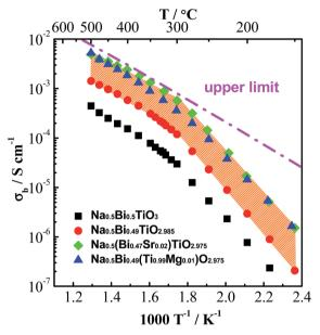
Fig. 5 An Arrhenius plot of bulk conductivity,  $\sigma_{\rm b}$ , for undoped and acceptor-doped NBT ceramics.41 The dash-dot line represents the upper limit of  $\sigma_b$  based on the oxygen-vacancy diffusion coefficient predicted in ref. 45, see text.
