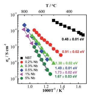
Fig. 8 Arrhenius plot of the bulk conductivity,  $\sigma_{\rm b}$ , of Nb-doped NBT with a nominal composition  $Na_{0.5}Bi_{0.5}Ti_{1-x}Nb_xO_{3+0.5x}$ . Activation energy for each composition is indicated in the figure. Replotted after ref. 29 and 34.
