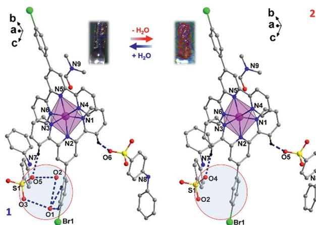
Fig. 1 Asymmetric units of **1** and **2**. Hydrogen atoms have been omitted for clarity. The purple dashed lines represent H-bonds. The two water molecules in the circle were removed through dehydration.
