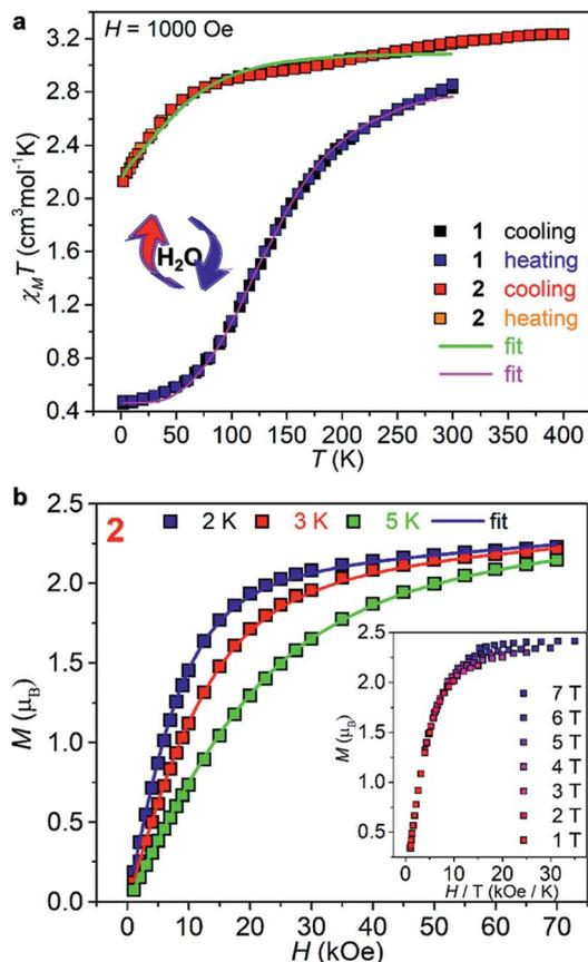
Fig. 2 (a) Susceptibility temperature product  $\chi T$  as a function of temperature (2–400 K) recorded on powder samples of **1** and **2** at an applied field of 1000 Oe. (b) Magnetization as a function of applied magnetic field at 2, 3, and 5 K for the same sample. The solid lines in (a) and (b) are spin Hamiltonian fits. Inset: reduced magnetization data of **2** collected in the temperature range of 2–10 K under applied dc fields of 1–7 T.
