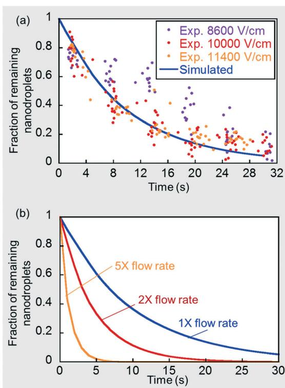
Fig. 7 (a) Simulation of the convection-controlled scenario and comparison to experimental results under a CP flow rate of 50  $\mu\text{L min}^{-1}$  and DP flow rate of 10  $\mu\text{L min}^{-1}$ . (b) Convection-controlled simulation results at 5 $\times$ , 2 $\times$ , and 1 $\times$  of the base flow rate of 50  $\mu\text{L min}^{-1}$  (CP) and 10  $\mu\text{L min}^{-1}$  (DP).
