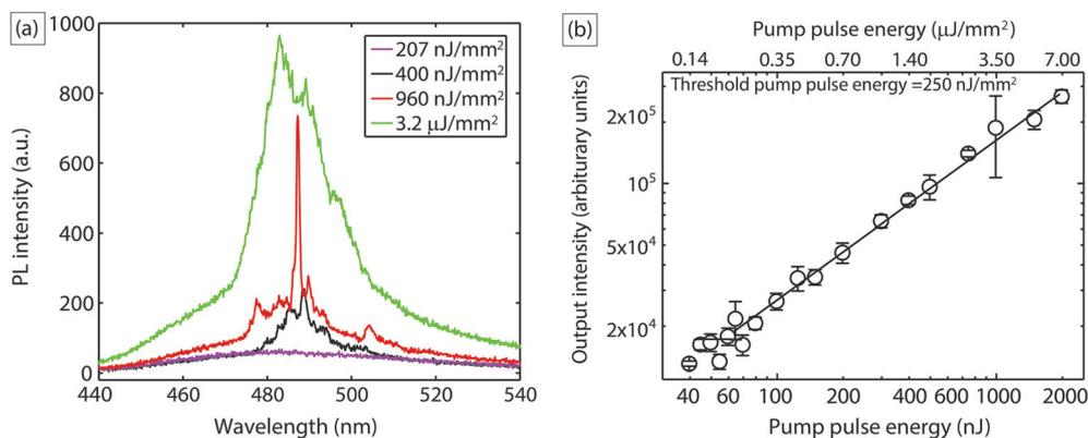
**Fig. 5** (a) Spectra obtained from wrapped laser shells at pump energies below and above the lasing threshold. (b) Nonlinear dependence of lasing emission intensity on pump pulse energy. Error bars represent standard deviation obtained from 10 consecutive droplets.
