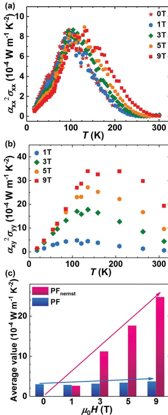
Fig. 2 The power factor PF  $\alpha_{xx}^2 \sigma_{xx}$  (a), Nernst power factor  $\text{PF}_{\text{Nernst}}$   $\alpha_{xy}^2 \sigma_{yy}$  (b) and average values of PF and  $\text{PF}_{\text{Nernst}}$  over the investigated temperature range (c) for polycrystalline NbP under different magnetic fields.
