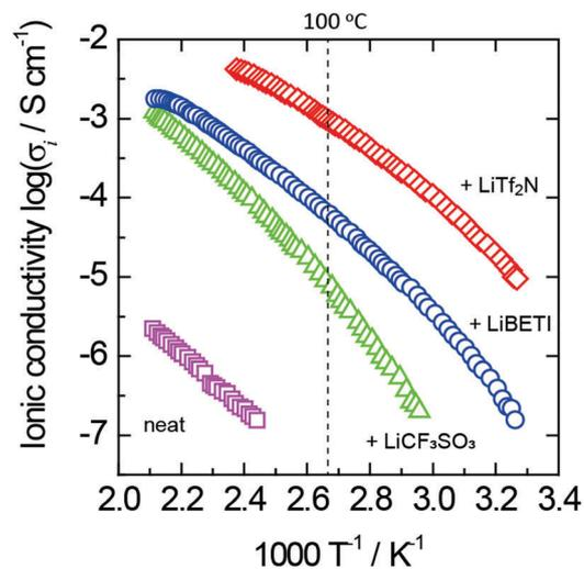
Fig. 4 Arrhenius plots of ionic conductivity for neat **1** and its lithium-salt complexes. The lithium-salt content is 50 mol% for all the complexes.
