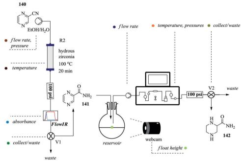
Multi-step semi continuous flow synthesis of piperazine-2-carboxamide.
