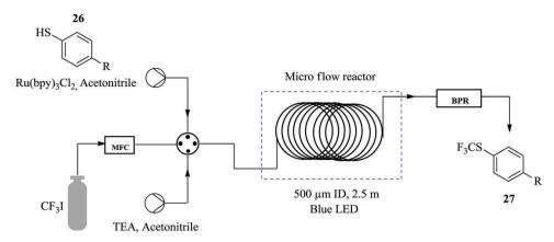
Fig. 2 Continuous flow photocatalytic trifluoromethylation of thiols
