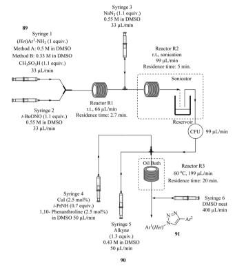
Fig. 11 A telescoped 3-step process for the synthesis of triazoles via diazotization, azidodediazotization and copper catalysed alkyne-azide cycloaddition.
