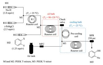
Fig. 16 Continuous flow synthesis of functionalized phenols.
