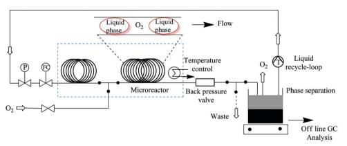
Fig. 6 Continuous flow set up for oxazole methyl alcohol synthesis with liquid recycle-loop
