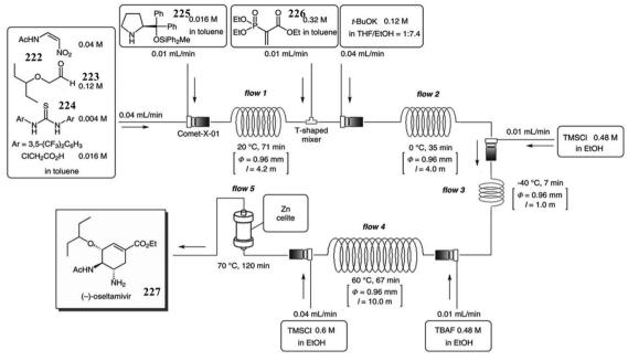
Fig. 27 Multi-step continuous flow synthesis of (-)-oseltamativir.
