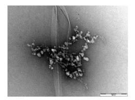
Fig. 7 TEM image of DBS-COOH gel (0.2% w/v) in the presence of heparin (38 μM) and C16-DAPMA (150 μM). Scale bar: 200 nm.
