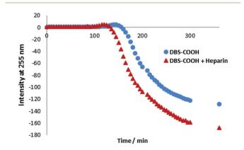
Fig. 2 CD intensity at 255 nm plotted against time for DBS-COOH (0.02% wt/vol) in the absence and presence of heparin (38  $\mu$ M).
