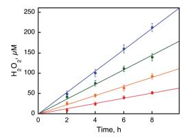
Fig. 4 Time courses of the photocatalytic production of  $H_2O_2$  from  $H_2O$  and  $O_2$  with  $[Ru^{II}(Me_2phen)_3]^{2^+}$  (0.10 mM) in the presence of a catalytic amount of 1 [0.50 mM (red), 1.0 mM (orange), 1.5 mM (green), and 2.0 mM (blue)] in an air-saturated solvent mixture of MeCN and  $H_2O$  (v/v =23:2) containing Sc(NO $_3$ ) $_3$  (100 mM) under photoirradiation (white light) at 298 K.
