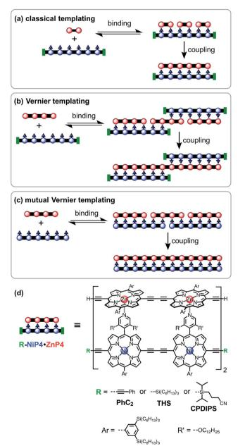
Fig. 1 Linear template-directed syntheses of monodisperse linear porphyrin oligomers. (a) Classical template-directed synthesis. (b) Vernier templating synthesis. (c) Mutual Vernier templating: both strands couple. (d) Key to molecular design.
