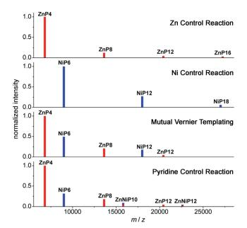
Fig. 13 Schematic of MALDI-TOF spectra of the mutual Vernier templating and three control reactions of the synthesis of NiP12 and ZnP12. Red lines represent the zinc porphyrin oligomers while blue lines indicate the nickel porphyrin oligomers. The mixed red-blue color indicates the heterocoupling zinc–nickel porphyrin oligomers. (See Fig. S34–S37† for raw mass spectra.)
