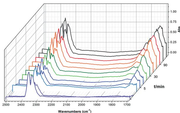
Fig. 3 *In situ* FT-IR spectra of the synthesis of chloropropene carbonate catalyzed by 2 at 100 °C under an atmospheric dilute CO<sub>2</sub>/N<sub>2</sub> gas mixture. IR absorption of 2 is subtracted for clarity.
