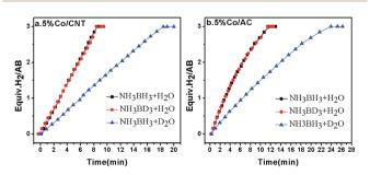
Fig. 1 Hydrogen evolution from NH<sub>3</sub>BH<sub>3</sub> in H<sub>2</sub>O (black), NH<sub>3</sub>BD<sub>3</sub> in  $H_2O$  (red), and  $NH_3BH_3$  in  $D_2O$  (blue) catalyzed by 5% Co/CNT (left) and 5% Co/AC (right) at room temperature,  $n_{Co}$ :  $n_{AB} = 0.05$ : 1.
