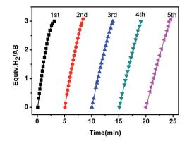
Fig. 5 The plots of volume of  $H_2$  vs. time for hydrolysis of AB catalyzed by the 5% Co/CTF-1 catalyst during a five-cycle reusability test.
