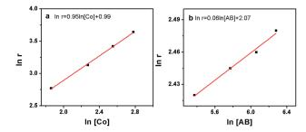
Fig. 4 (a) The plot of hydrogen generation rate *versus* the concentration of Co both in natural logarithmic scale, ln(rate) = 0.95 ln[Co] + 0.99; (b) the plot of hydrogen generation rate *versus* the concentration of AB both in natural logarithmic scale, ln(rate) = 0.06 ln[AB] + 2.07.
