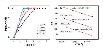
Fig. 7 (a) Plots of volume of  $H_2$  vs. time for the 5% Co/CTF-1 catalyzed hydrolysis of AB at temperatures in the range of 298-313 K, catalyst/AB = 0.05; (b) Arrhenius plots obtained from the kinetic data of 5% Co/ CTF-1, 5% Co/CNT, and 5% Co/AC
