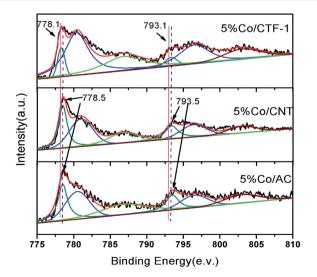
Fig. 6 XPS spectra of Co  $2p_{3/2}$  and  $2p_{1/2}$  in 5% Co/CTF-1, 5% Co/CNT and 5% Co/AC samples. All samples were pre-treated with Ar sputtering.
