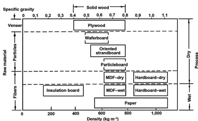
**Fig. 1** Classification of wood-based panels.<sup>17</sup>**Table 2** Advantages and disadvantages of synthetic adhesives used in manufacturing of WBPs<sup>9</sup>
