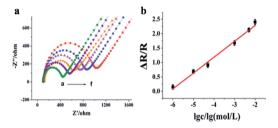
Fig. 31 (a) Impedance spectra of the PMAH/CNTs-NFs/GCE as a function of formaldehyde concentration [(a) 1  $\mu mol~L^{-1}$ , (b) 10  $\mu mol~L^{-1}$ , (c) 50  $\mu mol~L^{-1}$ , (d) 3 mmol  $L^{-1}$ , (e) 5 mmol  $L^{-1}$ , (f) 10 mmol  $L^{-1}$ ] in 0.1 mol  $L^{-1}$  KCl containing 5 mmol  $L^{-1}$  [Fe(CN)<sub>6</sub>]  $^{3/4}$ . (b) Calibration curve for the electrospun sensor (this figure has been adapted from ref. 79 with permission from RSC).
