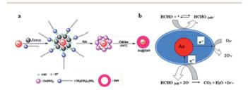
Fig. 26 (a) Schematic of the formation of Au@ZnO; (b) scheme for detection of FA (this figure has been adapted from ref. 77 with permission from Elsevier).
