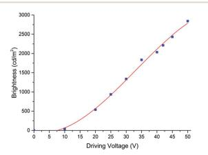
Fig. 4 Driving voltage – brightness characterization of the fully solution processed blue OLEC, measured at voltage pulse mode (30 ms pulse width, 1% duty cycle).
