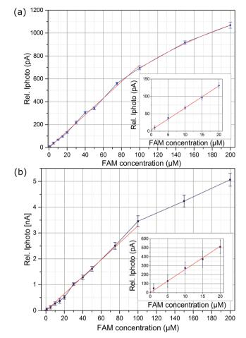
Fig. 8 Fluorescent detection measurement by integrated OLEC and OPD with different FAM dye concentration in water. The FAM solution was excited by the blue OLEC with brightness of (a)  $500 \text{ cd m}^{-2}$  and (b)  $2000 \text{ cd m}^{-2}$ ; the inset graph is the zoom-in of the low concentration part (1 to 20 μM).
