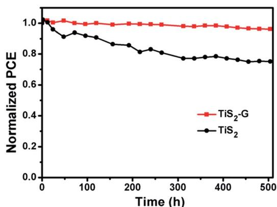
Fig. 30 Stability of DSSCs with TiS<sub>2</sub>–graphene hybrid and Pt CEs. Reprinted with permission from ref. 199, X. Meng, C. Yu, B. Lu, J. Yang and J. Qiu, dual integration system endowing two-dimensional titanium disulfide with enhanced triiodide reduction performance in dye-sensitized solar cells. *Nano Energy*, 2016, **22**, 59–69. Copyright© Elsevier.
