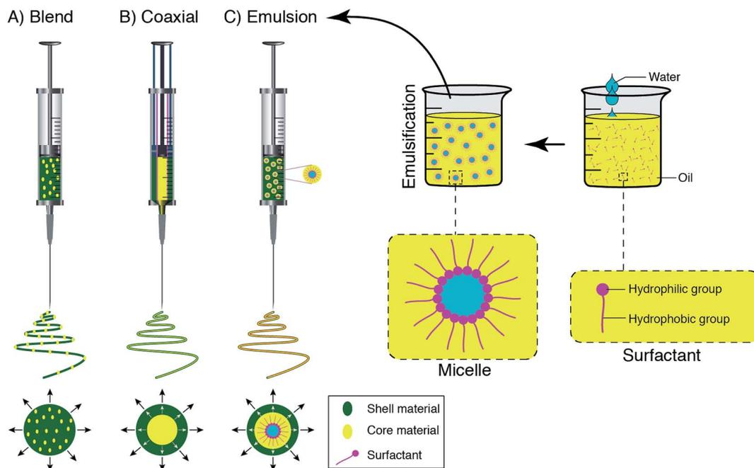
Fig. 3 Schematic displays of the spinneret loaded with a bioactive agent for (A) blend, (B) coaxial, and (C) emulsion electrospinning.
