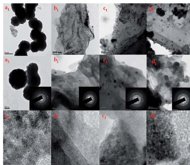
Fig. 4 HRTEM images of (a<sub>1</sub>–a<sub>3</sub>) MnS nanoparticles (b<sub>1</sub>–b<sub>3</sub>) MnS/G-9 (c<sub>1</sub>–c<sub>3</sub>) MnS/NG-9 and (d<sub>1</sub>–d<sub>3</sub>) MnS/BG-9 nanocomposites. Inset pictures shows SAED pattern of samples (a<sub>2</sub>–d<sub>2</sub>).
