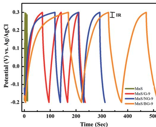
**Fig. 11** Galvanostatic charge/discharge behavior of MnS, MnS/G-9, MnS/NG-9 and MnS/BG-9 nanocomposite at a current density 0.5 A g<sup>-1</sup>.
