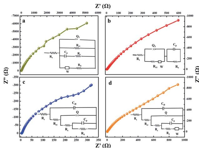
**Fig. 12** Nyquist plots of (a) pure MnS (b) MnS/G-9 (c) MnS/NG-9 and (d) MnS/BG-9 nanocomposite from the frequency range from 0.01 Hz to 10<sup>5</sup> Hz (inset shows the fitted equivalent circuits).
