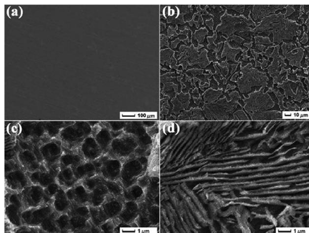
Fig. 4 Morphological images recorded via SEM clearly elucidate the differences for (a) the bare steel and (b) the textured steel surface. (c and d) Magnified images of (b).<sup>49</sup> Reprinted with permission from ref. 49. Copyright 2015, Elsevier B. V.
