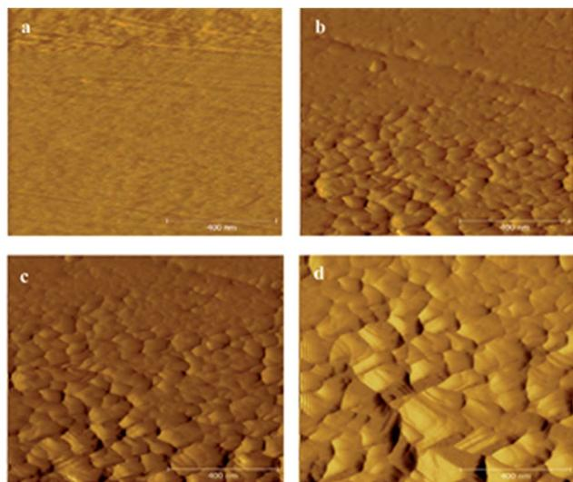
Fig. 7 *In situ* AFM topographical images of (a) untreated (bare) carbon steel before immersion, and in brine containing DPC (500 ppm) after (b) 5 min, (c) 30 min, and (d) 4 h immersion.<sup>83</sup> Reprinted with permission from ref. 83. Copyright 2014, American Chemical Society.
