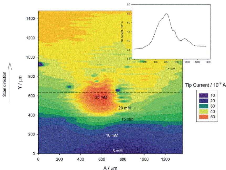
Fig. 20 SECM contour plot exhibiting defect in tin plate which was immersed in 10 mM  $\text{H}_2\text{SO}_4$ .  $E_{\text{tip}} = +600$  mV,  $E_{\text{sample}} = \text{OCP}$  (about 520 mV), SECM Pt tip radius = 10  $\mu\text{m}$ .<sup>168</sup> Reprinted with permission from ref. 168. Copyright 2006, Elsevier B. V.
