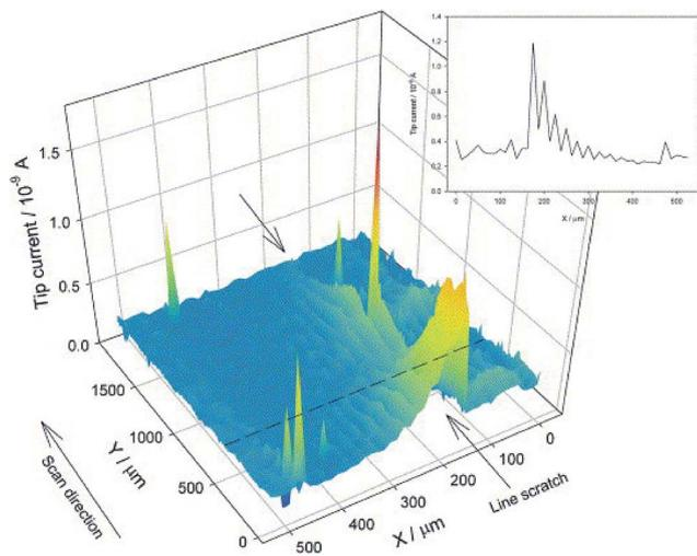
Fig. 19 SECM image of tinplate with a line scratch immersed in 10 mM  $\text{H}_2\text{SO}_4$ . The current increase above the scratch shows the oxidation of  $\text{Fe}^{2+}$  to  $\text{Fe}^{3+}$ .  $E_{\text{tip}} = +600$  mV,  $E_{\text{sample}} = \text{OCP}$  (about 520 mV), SECM Pt tip radius: 10  $\mu\text{m}$ .<sup>168</sup> Reprinted with permission from ref. 168. Copyright 2006, Elsevier B. V.
