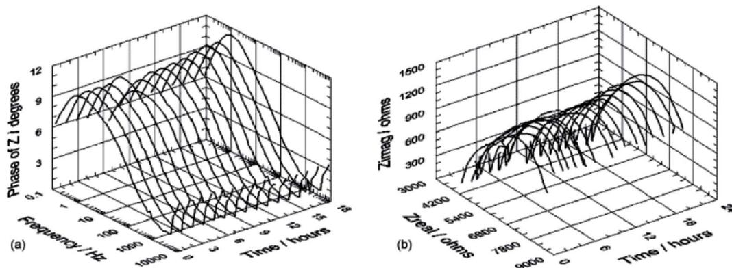
Fig. 11 *In situ* (a) EIS Bode phase angle and (b) complex-plane impedance plots data for a polished mild steel electrode immersed in 3% (w/v) NaCl saturated with high purity carbon dioxide at atmospheric pressure (adjusted to pH 4.75).<sup>90</sup> Reprinted with permission from ref. 90. Copyright 2007, Elsevier B. V.
