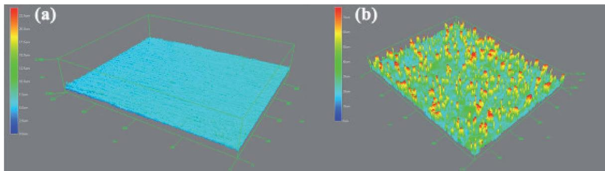
Fig. 5 Surface profile variations in (a) the bare steel and (b) the textured steel surface.<sup>49</sup> Reprinted with permission from ref. 49. Copyright 2015, Elsevier B. V.
