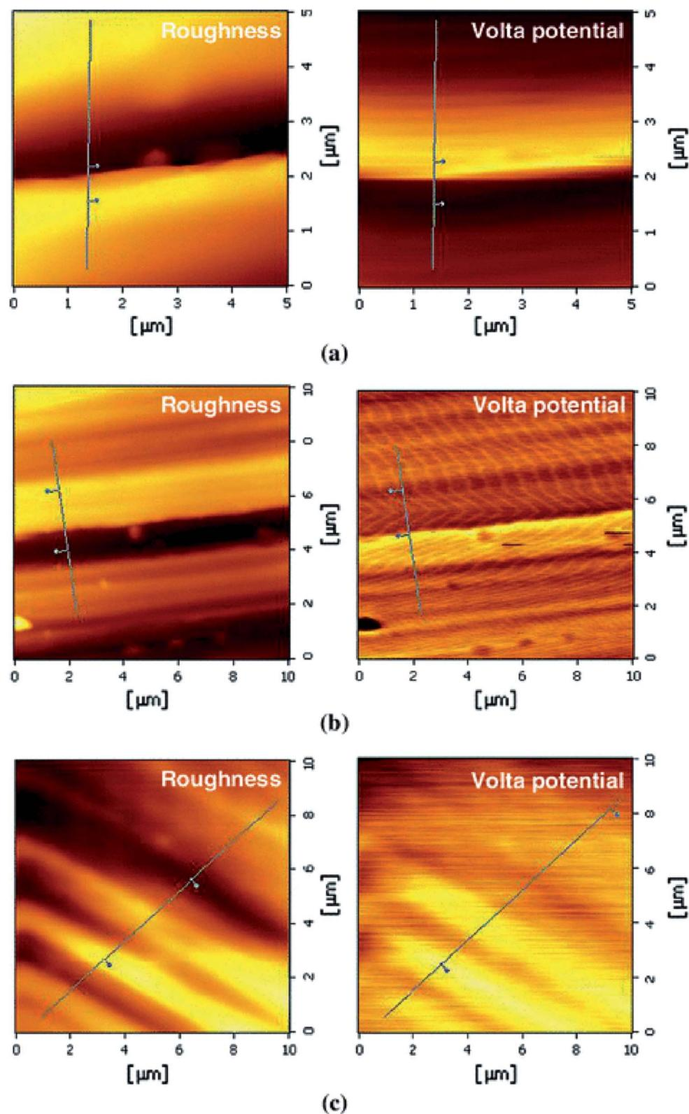
Fig. 16 KPFM image representing topography and Volta potential with different average roughness; (a) Ra 108.0 nm, (b) Ra 39.3 nm, and (c) Ra 16.7 nm.<sup>152</sup> Reprinted from ref. 152 with permission of Springer. Springer Science + Business Media Dordrecht 2013.
