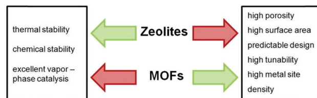
Fig. 6 Strengths (green) and weaknesses (red) of zeolites and MOFs, respectively. Modified from ref. 46.
