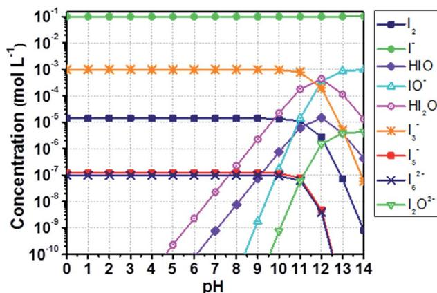
Fig. 1 Computed concentration of iodine compounds in a solution containing aqueous I<sup>-</sup> 0.10 M and I<sub>2</sub> 1.0 mM as a function of the pH. Results are computed as described in this section, comparable with those obtained by Gottardi (see Fig. S1†).<sup>31</sup> Lines just connect data points for better reading and have no physical meaning.
