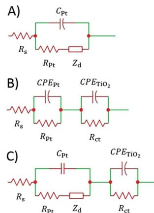
Fig. 2 Equivalent circuits proposed for the EIS investigation of aqueous devices under study.
