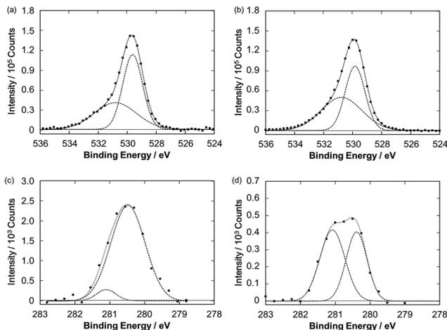
Fig. 7  $\circ$  1s XPS spectra of the Ru–ZnP/TiO<sub>2</sub>/FTO electrodes (a) before and (b) after the PEC operation. Ru 3d<sub>5/2</sub> XPS spectra of the Ru–ZnP/TiO<sub>2</sub>/FTO electrodes (c) before and (d) after the PEC operation.
