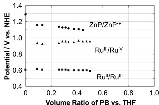
Fig. 2 Plots of the redox potential (V vs. NHE) of ZnP/ZnP<sup>•+</sup> (circle), Ru<sup>III/IV</sup> (triangle) and Ru<sup>II/III</sup> (square) as a function of the volume ratio of the PB/THF mixture for **Ru-ZnP**. The ratio was changed from 0 to 0.5. The electrochemical measurements for ratios >0.5 were unable to be conducted due to the aggregation in the mixed solvent.
