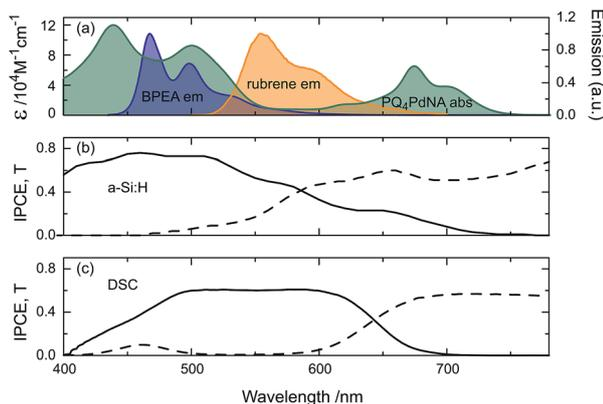
Fig. 3 The spectral properties of the two UC/device assemblies in this study: (a) absorption of PQ<sub>4</sub>PdNA (green) and emission of rubrene (orange) and BPEA (blue). IPCE (solid) and transmittance (dash) of (b) a-Si:H, illuminated through glass substrate and (c) DSC, illuminated through working-electrode.
