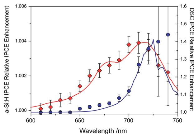
Fig. 5 Relative enhancement trace for a-Si:H device ( $\diamond$ , red trace) tested with  $\sim 1.4$  suns equivalent illumination ( $\lambda = 670 \pm 5$  nm) and a DSC ( $\circ$ , blue trace) tested with  $\sim 1.3$  suns equivalent illumination, including the modeled traces for the two devices.<sup>40,41</sup>
