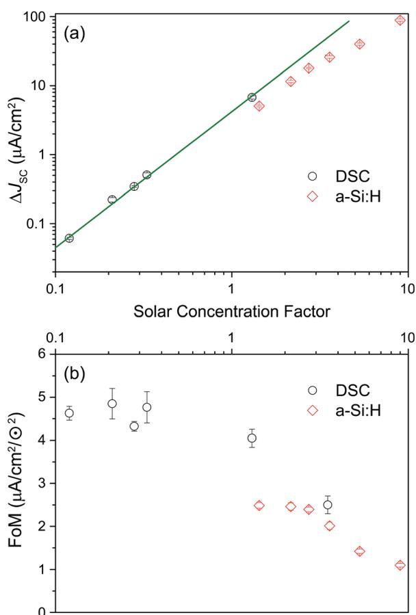
Fig. 6 (a) Dependence of calculated current gain ( $\Delta J_{SC}$ ) on effective solar concentration (both axes on a logarithmic scale) for the a-Si:H device ( $\diamond$ ) and DSC ( $\circ$ ). (b) Figure of merit (FoM) as a function of solar concentration for a-Si:H ( $\diamond$ ) and DSC ( $\circ$ ).
