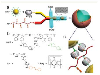
Fig. 2 (a) Schematic of the preparation of supramolecular colloidal microcapsules by a flow-focusing microfluidic device, consisting of a continuous FC-40 oil phase perpendicular to a combination of two aqueous solutions of MCPCCB[8] and AP as the dispersed phase. (b) Molecular structure of MCP, AP, and CB[8]. (c) Schematic representation of the proposed microcapsule from CB[8]-mediated supramolecular assembly.
