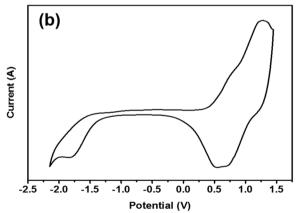
Fig. 3 (a) UV-vis absorption spectra at room temperature (dotted line drop cast thin film absorption on the quartz plate, thick line - dilute solution absorption in TCB), (b) cyclic voltammetric profile (in 0.1 M Bu<sub>4</sub>NPF<sub>6</sub> in dichloromethane as the supporting electrolyte with a scan rate of 100 mV s<sup>-1</sup> and the potentials reported are versus the Fc<sup>+</sup>/Fc redox couple as an external standard) of DTmBDT copolymer.
