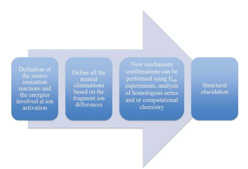
Fig. 33 Suggested steps for structural elucidation using MS fragmentation.
