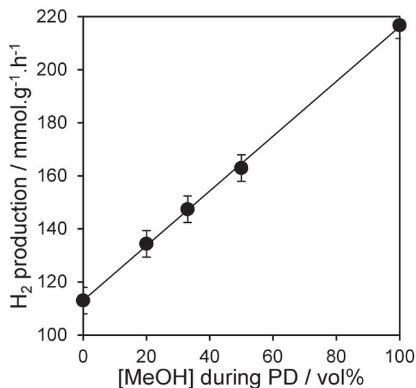
Fig. 1 Photocatalytic hydrogen evolution over 1 wt% Pt/TiO<sub>2</sub> catalysts as a function of methanol concentration during PD.
