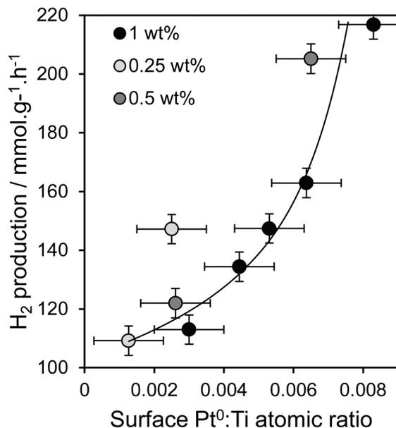
Fig. 10 Relationship between the rate of photocatalytic hydrogen production and dispersion of metallic Pt metal for Pt/TiO<sub>2</sub> catalysts prepared via PD.
