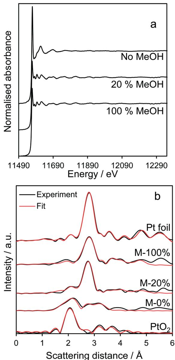
Fig. 6 Fluorescence Pt  $L_{III}$ -edge (a) normalized XANES spectra and (b) radial distribution functions of Pt/TiO<sub>2</sub> catalysts. Pt foil and oxide references shown for comparison.
