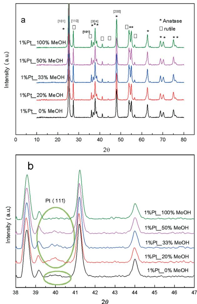
Fig. 2 (a) Wide angle and (b) high resolution XRD patterns of 1 wt% Pt/TiO<sub>2</sub> catalysts as a function of methanol concentration during PD.
