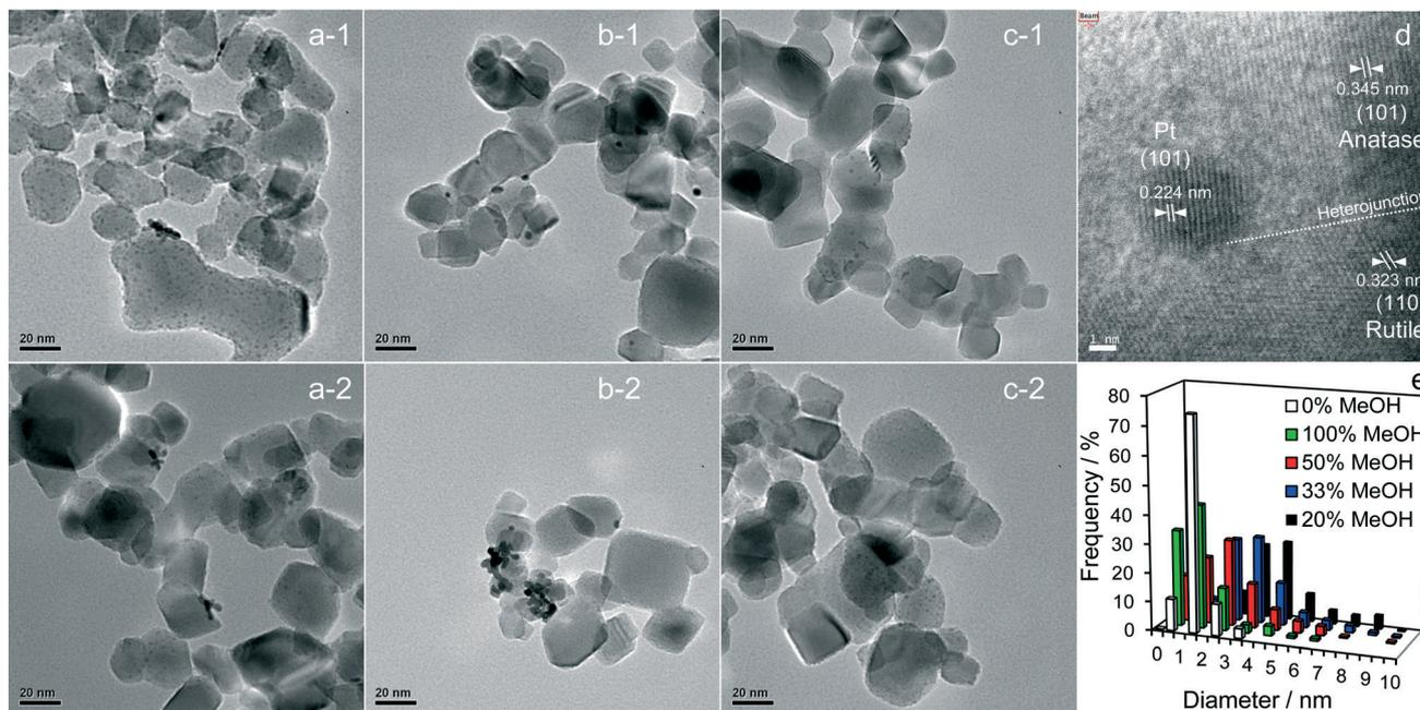
Fig. 3 Representative bright-field HRTEM images of (a1–2) 100%, (b1–2) 20%, and (c1–2) 0% MeOH 1 wt% Pt/TiO<sub>2</sub>, (d) an individual Pt metal nanoparticle at the interface between anatase and rutile crystallites, and (e) particle size distributions as a function of methanol concentration during PD.
