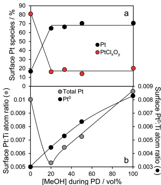
Fig. 5 (a) Evolution of platinum surface oxidation state, and (b) relative dispersion of total and metallic platinum for 1 wt% Pt/TiO<sub>2</sub> catalysts as a function of methanol concentration during PD.
