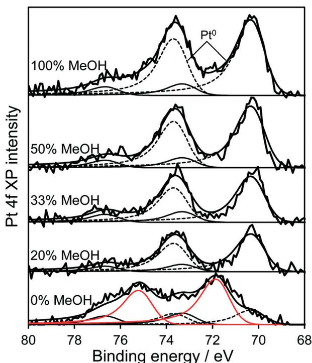
Fig. 4 Pt 4f XP spectra of 1 wt% Pt/TiO<sub>2</sub> catalysts as a function of methanol concentration during PD.
