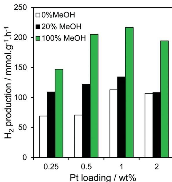
**Fig. 9** Photocatalytic hydrogen evolution over Pt/TiO<sub>2</sub> catalysts as a function of Pt loading and methanol concentration during PD.
