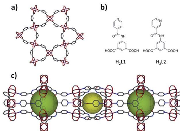
Fig. 1 (a) Layer segment of a **kgm-MOF**. (b) Left: 5-(isonicotinamido)isophthalic acid (H<sub>2</sub>L1) and right: 5-(nicotinamido)isophthalic acid (H<sub>2</sub>L2). (c) Hourglass-shaped channels with two primary types of cavities. C = gray, O = red, N = blue, Cu = plum; H atoms are omitted for clarity.
