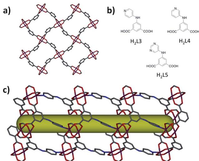
Fig. 2 (a) Layer segment of a **sql**-MOF. (b) Left, up: 5-(pyridin-4-ylamino)isophthalic acid ( $\text{H}_2\text{L}_3$ ). Right, up: 5-(pyridin-3-ylamino)isophthalic acid ( $\text{H}_2\text{L}_4$ ). Bottom: 5-(pyrimidin-5-ylamino)isophthalic acid ( $\text{H}_2\text{L}_5$ ). (c) Projection along the *a*-axis of the **rtl**-MOF-**2** displaying channel. C = gray, O = red, N = blue, and Cu = plum; H atoms are omitted for clarity.
