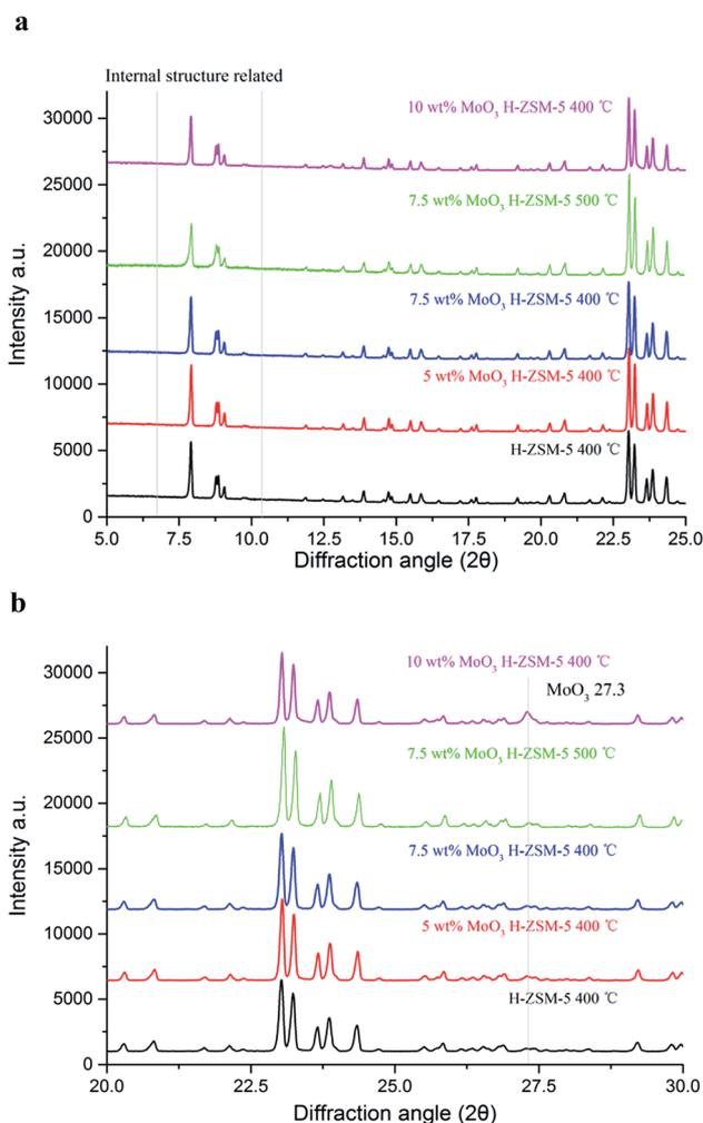
Fig. 2 (a) X-ray diffraction patterns (2θ = 5–25°) of MoO<sub>3</sub>/ZSM-5 samples with various MoO<sub>3</sub> loadings and prepared at 400 °C/500 °C. (b) X-ray diffraction patterns (2θ = 20–30°) of MoO<sub>3</sub>/ZSM-5 samples with various MoO<sub>3</sub> loadings and prepared at 400 °C/500 °C.
