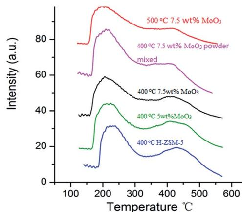
Fig. 6  $\text{NH}_3$ -temperature programmed desorption profiles of  $\text{MoO}_3$ /H-ZSM-5 samples prepared via different conditions (impregnation/powder mixing,  $400$ – $500\text{ }^\circ\text{C}$ ) together with the original H-ZSM-5 sample ( $400\text{ }^\circ\text{C}$ ).
