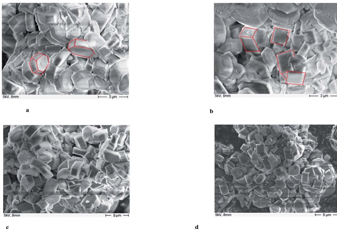
Fig. 7 (a) SEM image of the parent H-ZSM-5. (b) SEM image of H-ZSM-5 with 7.5 wt% MoO<sub>3</sub>-400 °C dispersion. (c) SEM image of the parent H-ZSM-5 (post reaction). (d) SEM image of H-ZSM-5 with 7.5 wt% MoO<sub>3</sub>-400 °C (post reaction).
