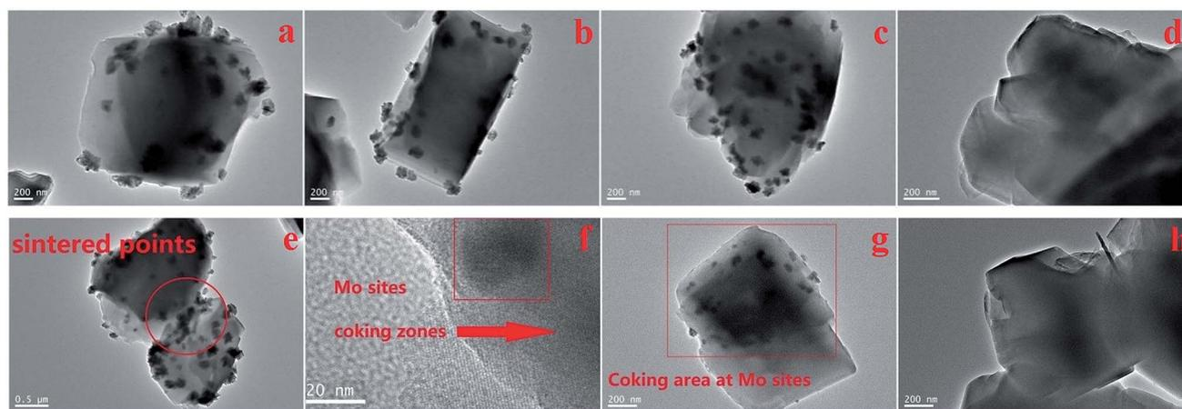
Fig. 8 TEM images of post catalytic-testing samples with different MoO<sub>3</sub> loadings, (a) 5 wt%, (b) 7.5 wt%, (c) 10 wt% and (d) parent H-ZSM-5, (e) sintering effects (5 wt%), (f) amplified coking areas near the Mo species (5 wt%), (g) coking areas near Mo species (5 wt%) and (h) parent H-ZSM-5, all the samples are prepared at 400 °C and the MTH reaction proceeded at 400 °C. More images of other samples are included in the Fig. S1–S9.†
