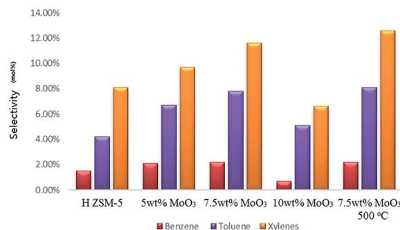
**Fig. 9** Selectivity to benzene, toluene and xylenes after a 5 h catalytic run; WHSV = 2 h<sup>-1</sup>, catalyst bed temperature 400 °C, and atmosphere pressure conditions.
