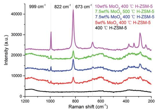
Fig. 3 Laser Raman spectra of the as prepared MoO<sub>3</sub>/ZSM-5 samples and H-ZSM-5 and prepared at 400 °C/500 °C.
