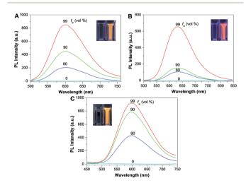
Fig. 2 Fluorescence spectra of TPDC (A), TPPDC (B), PPDC (C) in DMSO/water mixtures with different volume fractions of water at a concentration of 10  $\mu M$ . The excitation wavelengths for (A), (B) and (C) are 400, 390, 420 nm, respectively. The insets show photographs of the compounds in DMSO and DMSO : water (v : v, 1 : 99) under UV light (365 nm) illumination.
