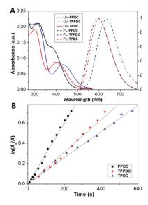
Fig. 3 (A) UV-vis absorption (solid lines) and normalized photo-luminescence (PL) spectra (dashed lines) of 10  $\mu$ M each of PPDC, TPDC and TPPDC in DMSO/water (v/v = 1/99). (B) The decomposition rates of ABDA by PPDC, TPDC and TPPDC;  $A_0$  and A are the absorbance of ABDA in the presence of the AlEgen PSs at 378 nm before and after irradiation, respectively.
