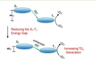
Scheme 1 A physical model of  $^1O_2$  generation, depicting the  $S_1-T_1$  ISC process and the proposed strategy for increasing  $^1O_2$  generation.
