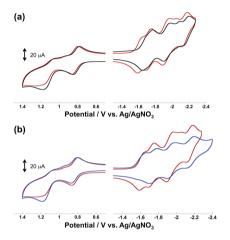
Fig. 4 Cyclic voltammograms of (a) Ru(CH2OCH2)Re (red) and Ru(CH<sub>2</sub>CH<sub>2</sub>CH<sub>2</sub>)Re (black), and (b) Ru(CH<sub>2</sub>SCH<sub>2</sub>)Re (blue) and Ru(CH<sub>2</sub>OCH<sub>2</sub>)Re (red) measured in MeCN containing Et<sub>4</sub>NBF<sub>4</sub> (0.1 M) as the supporting electrolyte.
