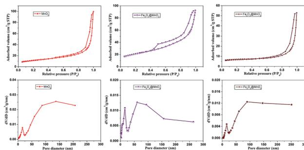
Fig. 4 The nitrogen adsorption–desorption isotherms and pore size distributions of as-prepared  $\text{MnO}_2$ ,  $\text{Fe}_3\text{O}_4@MnO_2$  and  $\text{Fe}_2\text{O}_3@MnO_2$  nanocomposites samples at time of 6 h calculated by BJH method.
