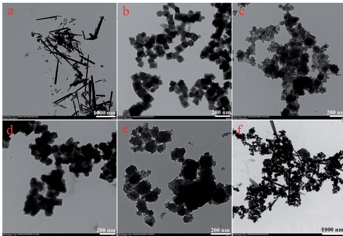
Fig. 2 TEM images of as-prepared nanostructures. (a),  $\text{MnO}_2$ ; (b),  $\text{Fe}_3\text{O}_4$ ; (c)–(f),  $\text{Fe}_3\text{O}_4@\text{MnO}_2$  nanocomposites prepared at times of 3 h, 6 h, 9 h, and 15 h, respectively.
