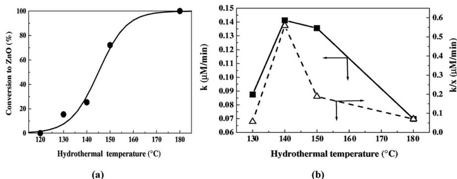
Fig. 15 (a) Phase transformation from ZnO<sub>2</sub> to ZnO; (b) rate constant (*k*) and normalized rate constant (*k*/*x*) vs. hydrothermal temperature (*x* is the ZnO<sub>2</sub>-to-ZnO conversion) for the degradation of MO (reprinted with permission from ref. 242; Copyright 2005 @ Elsevier).
