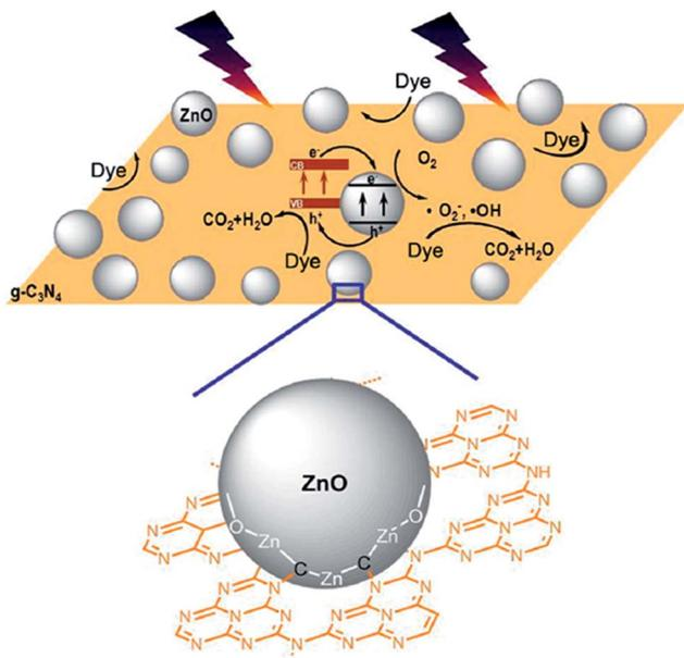
Fig. 24 Illustration of the electron–hole separation, transport, and photocatalytic progress of C–ZnO:g-C<sub>3</sub>N<sub>4</sub> under visible light (reprinted with permission from ref. 310; Copyright 2014 @ American Chemical Society).
