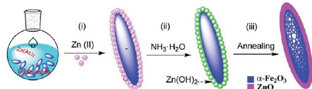
Fig. 17 Stepwise formation of a  $\text{Fe}_2\text{O}_3$ @ZnO heterostructure; (i) adsorption of zinc species on hematite seeds; (ii) addition of ammonia to form  $\text{Zn}(\text{OH})_2$ ; (iii) decomposition of the  $\text{Zn}(\text{OH})_2$  to form a ZnO layer (reprinted with permission from ref. 253; Copyright 2012 @ American Chemical Society).
