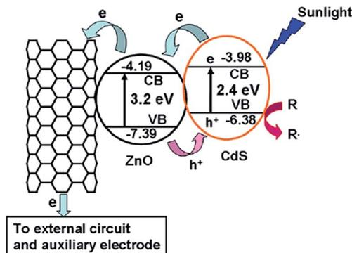
Fig. 25 Charge carrier separation and transportation in a CdS–ZNWs–MWCNTs heterojunction (reprinted with permission from ref. 311; Copyright 2011 @ Elsevier).
