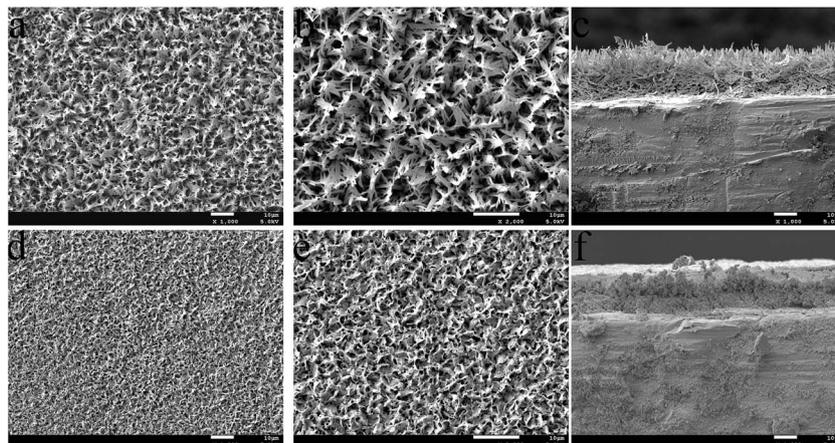
Fig. 2 SEM images of the (a and b) HAP coating and the (d and e) ZnCuHAP coating; Cross-section morphology of the (c) HAP coating and the (f) ZnCuHAP coating.
