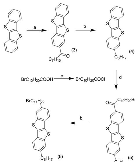
**Scheme 1** Synthetic route to molecule 6. (a) 1.1 eq. C<sub>7</sub>H<sub>15</sub>COCl, 2.5 eq. AlCl<sub>3</sub>, dry DCM, Ar, –78 °C, 4 h, 98%. (b) 2.5 eq. AlCl<sub>3</sub>, 2.5 eq. 1 M LiAlH<sub>4</sub> in Et<sub>2</sub>O, Ar, dry Et<sub>2</sub>O and DCM, rt, O/N, 100/98%. (c) 1.4 eq. oxalyl chloride, cat. DMF, Ar, dry DCM, 1 h, 100%. (d) 2.5 eq. AlCl<sub>3</sub>, dry DCM, Ar, –78 °C, 4 h, 88%.
