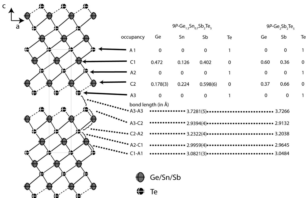
**Fig. 7** Atom distribution (occupancy factors, missing esd's are a consequence of constraints) for each element and bond lengths in the refined model of Ge<sub>1.3</sub>Sn<sub>0.7</sub>Sb<sub>2</sub>Te<sub>5</sub> at 293 K (displacement ellipsoids drawn at 99% probability level) compared with Ge<sub>2</sub>Sb<sub>2</sub>Te<sub>5</sub>.<sup>24</sup>
