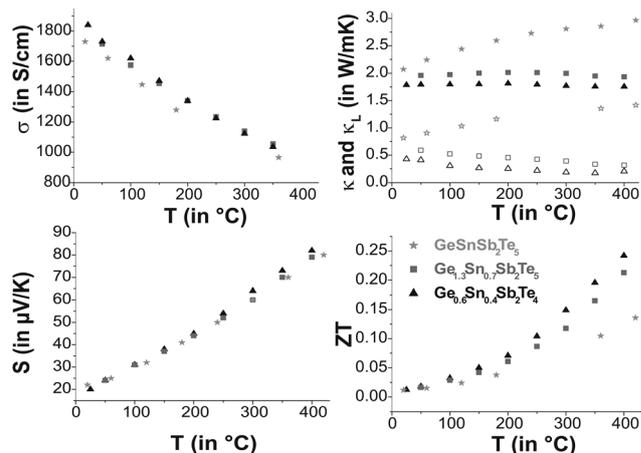
**Fig. 9** Thermoelectric properties of  $\text{Ge}_{0.6}\text{Sn}_{0.4}\text{Sb}_2\text{Te}_4$ ,  $\text{Ge}_{1.3}\text{Sn}_{0.7}\text{Sb}_2\text{Te}_5$  and  $\text{GeSnSb}_2\text{Te}_5$ : electrical conductivity and Seebeck coefficient (left side top to bottom); lattice thermal conductivity ( $\kappa$  bold and  $\kappa_L$  open faced) and thermoelectric figure of merit (right side top to bottom).
