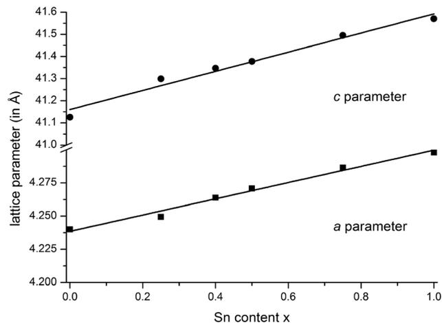
Fig. 1 Vegard's plot of compounds in the series  $(\text{Ge}_{1-x}\text{Sn}_x)\text{Sb}_2\text{Te}_4$  ( $x = 0-1$ ); c parameter (top) and a parameter (bottom); values for  $\text{GeSb}_2\text{Te}_4$ <sup>25</sup> and  $\text{SnSb}_2\text{Te}_4$ <sup>23</sup> taken from literature.
