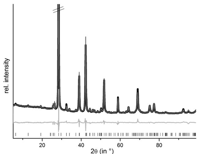
Fig. 2 Rietveld refinement of  $21R$ - $\text{Ge}_{0.5}\text{Sn}_{0.5}\text{Sb}_2\text{Te}_4$  (the strongest reflection is cut off); vertical lines indicate calculated reflection positions, experimental (black) and calculated pattern (gray) and difference plot (below) are shown.
