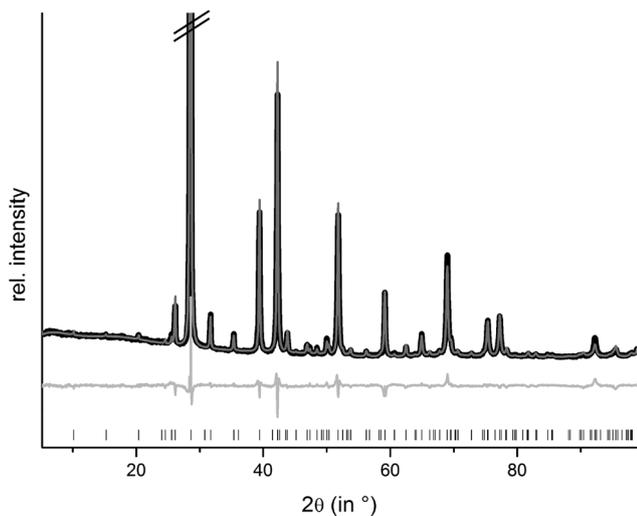
Fig. 6 Rietveld refinement of 9P-GeSnSb<sub>2</sub>Te<sub>5</sub>; (the strongest reflection is cut off); vertical lines indicate calculated reflection positions, experimental (black) and calculated pattern (gray) and difference plot (below) are shown.
