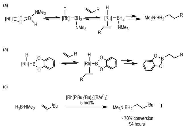
**Scheme 1** Rh-catalysed hydroboration using amine–borane (a) and catechol borane (b); hydroboration of TBE using H<sub>3</sub>B·NMe<sub>3</sub>, (c).
