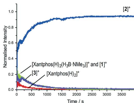
Fig. 3 ESI-MS under PSI conditions<sup>29</sup> of the reaction of TBE with  $\text{H}_3\text{B}\cdot\text{NMe}_3$  catalysed by 3. Conditions:  $\text{H}_3\text{B}\cdot\text{NMe}_3$ , 0.006 M, TBE 0.013 M; [3] 0.001 M, 1,2- $\text{F}_2\text{C}_6\text{H}_4$ . Under these conditions of concentration and experiment catalysis proceeded to 80% conversion.
