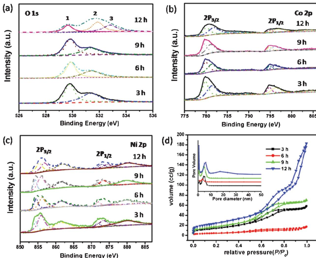
Fig. 6 (a–c) XPS spectra of NiCo<sub>2</sub>O<sub>4</sub> samples at 180 °C from different hydrothermal reaction times; (d) N<sub>2</sub> adsorption/desorption isotherms of NiCo<sub>2</sub>O<sub>4</sub> samples with corresponding pore-size distribution (inset).
