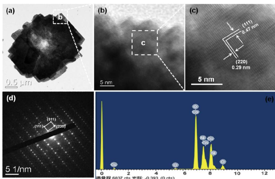
Fig. 5 (a–e) TEM, HRTEM images, SAED pattern and the EDS spectrum of  $\text{NiCo}_2\text{O}_4$  hierarchical flower-like super-structures consisting of porous  $\text{NiCo}_2\text{O}_4$  nanosheets.
