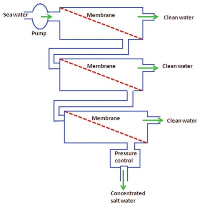
Fig. 4 Modules of connecting membranes in series.
