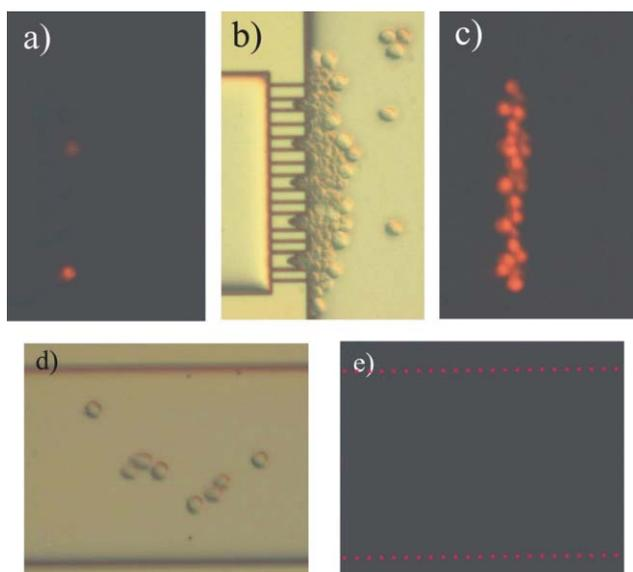
**Fig. 5** PI uptake in HL60 cells sitting at the trap due to the high electric field lines density. (a) Fluorescence image at the time the HL60 cells arrive at the trap. (b) Light microscopy image of the cells 10 s after EOF control was stopped. (c) Fluorescence image from image (b). (d) Light microscopy image of the central channel (R1). (e) Fluorescence image from image (d).
