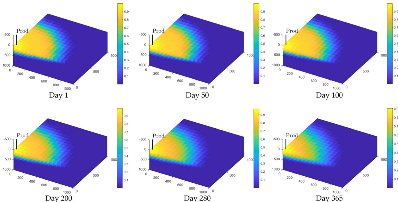
Fig. 6 Variation of hydrogen concentration during the production phase. The colour bar represents the hydrogen concentration.
