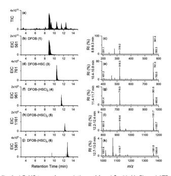
Fig. 2 LC-MS traces from solutions of  $\bf 1$  and  $\bf 2$  with MgCl<sub>2</sub> and ATP, incubated (37 °C, 2 h, pH 8) in the presence of StDesD, as detected by TIC (a), or shown as an EIC with values set to report the  $[M + H]^+$  adducts of (b)  $\bf 1$ , (d)  $\bf 3$ , (f)  $\bf 4$ , (h)  $\bf 5$ , or (j)  $\bf 6$ , with signature regions of the MS fragmentation pattern aligned at right (c, e, g, i and k).
