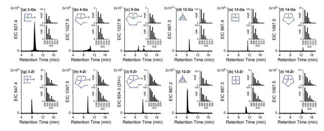
Fig. 5 EIC traces from biocombinatorial mixtures of chelators acquired following the addition of excess Ga(III) or Zr(IV) with EIC values set to report complexes between Ga(III) (a-f) or Zr(IV) (g-l) and 3-5, or 12-14, with isotope patterns (upper: experiment; lower: calculated) from the major or asterisked peak in the inset, and the relevant species as a cartoon.
