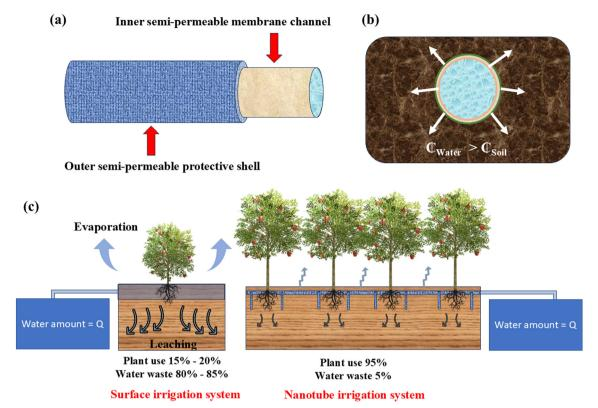
Fig. 5 (a) Internal structure of Moistube, 169 (b) water flow from Moistube to the surrounding soil, depending on soil water potential, and (c) irrigation water use efficiency of Moistube compared to the conventional surface drip irrigation system.
