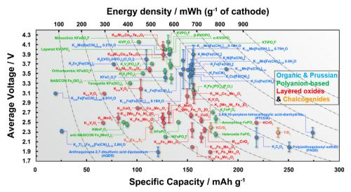
Ragone plots of representative cathode materials for potassium ion batteries. Figure adapted from ref. 114 with permission.
