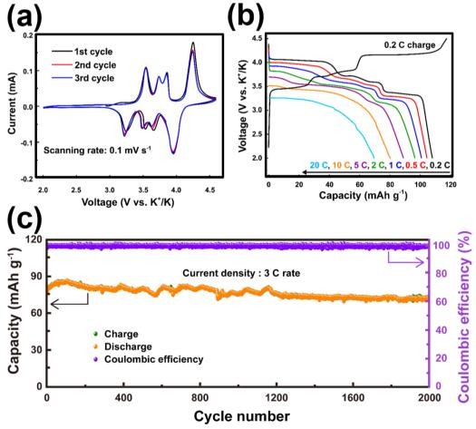
Fig. 15 Electrochemical performance of KFeSO<sub>4</sub>F. (a) Cyclic voltammogram of KFeSO<sub>4</sub>F taken at a scanning rate of 0.1 mV s<sup>-1</sup>. (b) Rate performance of KFeSO<sub>4</sub>F and (c) cycle performance at a current density commensurate to 3C. The theoretical capacity for KFeSO<sub>4</sub>F is 127.6 mA h g<sup>-1</sup> (1C = 127.6 mA g<sup>-1</sup>). Figures reproduced from ref. 14 with permission. Copyright 2022 Elsevier.
