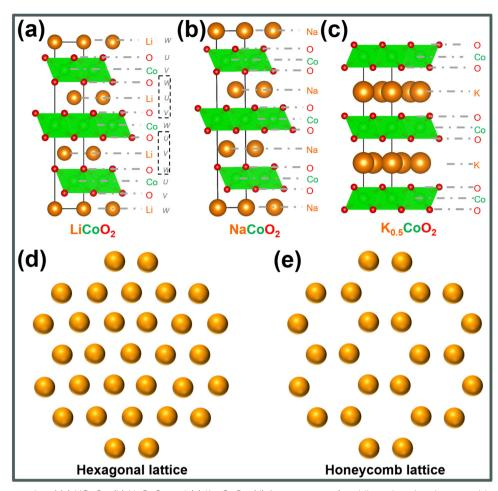
Fig. 18 Layered frameworks of (a) LiCoO<sub>2</sub>, (b) NaCoO<sub>2</sub> and (c) K<sub>0.5</sub>CoO<sub>2</sub>. (d) Arrangement of mobile cations in a hexagonal lattice as exemplified in LiCoO2 and NaCoO2. (e) Arrangement of mobile cations in a honeycomb lattice as exemplified in potassium-deficient K<sub>0.5</sub>CoO2.
