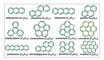
Fig. 10 Representative polycyclic aromatic hydrocarbons (including supertriphenylene, <sup>143</sup> superphenalene <sup>143,144</sup> and circumcoronene <sup>145,146</sup>), which can operate at high voltages via the insertion/extraction of anions such as PF<sub>6</sub><sup>-</sup>, BF<sub>4</sub><sup>-</sup>, FSI<sup>-</sup>, TFSI<sup>-</sup>, etc.
