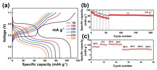
Fig. 31 Electrochemical performance of an all-solid-state potassium battery setup comprising Prussian blue K<sub>x</sub>Fe[Fe(CN)<sub>6</sub>] as cathode, K-C composite as the anode and  $\beta/\beta'' - Al_2O_3$  as solid electrolyte. (a) Voltage-capacity profiles at various current densities. (b) Cycle performance at various current densities. (c) Cycle performance at various temperature ranges. Figures reproduced with permission. 439 Copyright 2023 Wiley-VCH.
