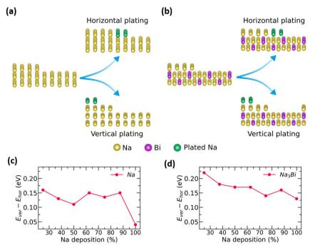
Fig. 5 Schematic representation illustrating the horizontal and vertical plating mechanisms of Na on (a) bulk Na-metal and (b) Na<sub>3</sub>Bi surfaces. The graphs below show the variation in the energy difference between vertical and horizontal plating in response to varying Na deposition concentrations for (c) bulk Na-metal and (d) Na<sub>3</sub>Bi surfaces.
