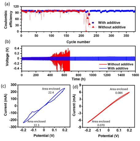
Fig. 4 (a) Coulombic efficiency of Na//Cu half cells with and without an additive at 1 mA cm<sup>-2</sup> current density and 1 mA h cm<sup>-2</sup> capacity. (b) Stripping plating cycling performance of a Na//Na symmetric cell at 1 mA cm<sup>-2</sup> current density and 1 mA h cm<sup>-2</sup> capacity, and the cyclic voltammogram of a Na//Na symmetric cell (c) with and (d) without an additive. The CV scans were conducted at a sweep rate of 5 mV s<sup>-1</sup>.
