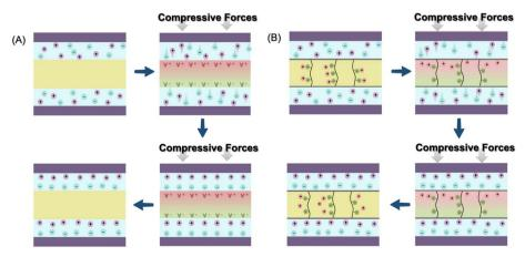
Fig. 4 Schematic illustration of the proposed mechanism for piezo-electrochemical (A) and piezo-ionic (B) processes
