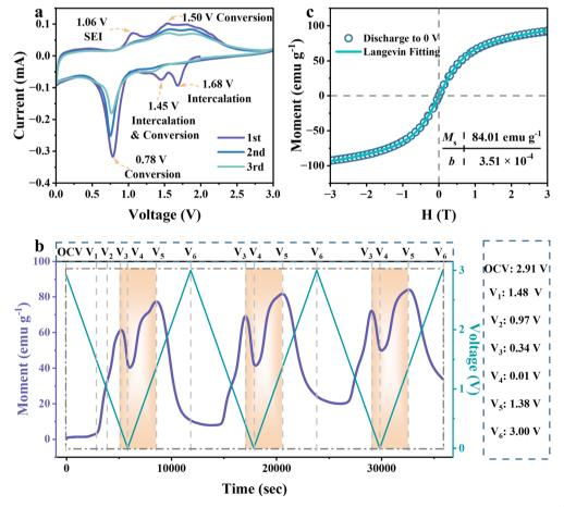
Fig. 2 Electrochemical reaction mechanism of FeOOH LIBs. (a) CV curves for the first three cycles at a scan rate of  $0.5~\text{mV}~\text{s}^{-1}$  over the voltage range of 0.01-3 V. (b) Operando magnetic monitoring followed the voltage range of CV scanning under a magnetic field of 3 T. (c) Magnetic hysteresis loop with the Langevin fitting curve after the first full discharge measured at 300 K.
