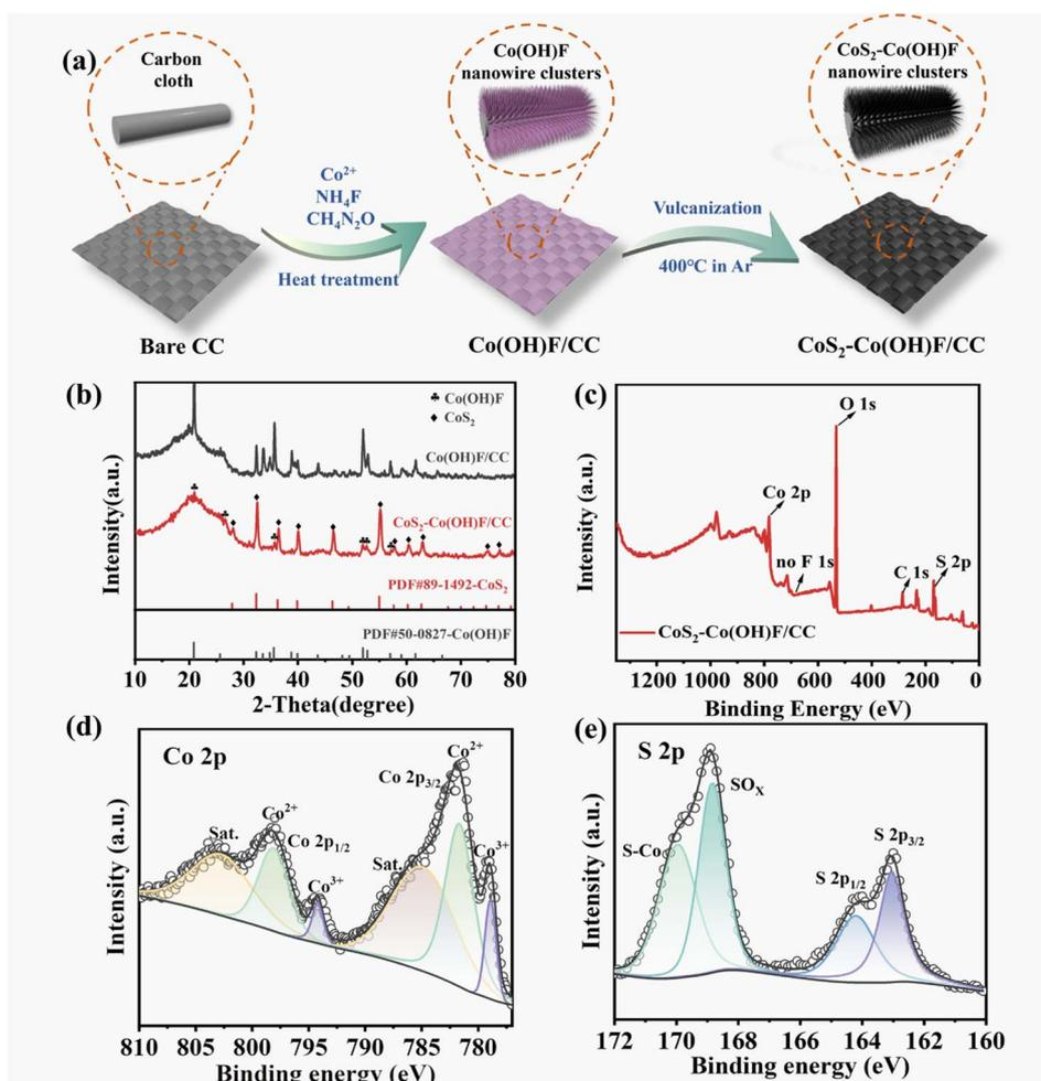
Fig. 1 (a) Schematic illustration showing the preparation of the  $\text{CoS}_2\text{-Co(OH)F}$  composite on the surface of CC. (b) XRD pattern and XPS spectra of the  $\text{CoS}_2\text{-Co(OH)F}$ : (c) full, (d) Co 2p and (e) S 2p spectra.
