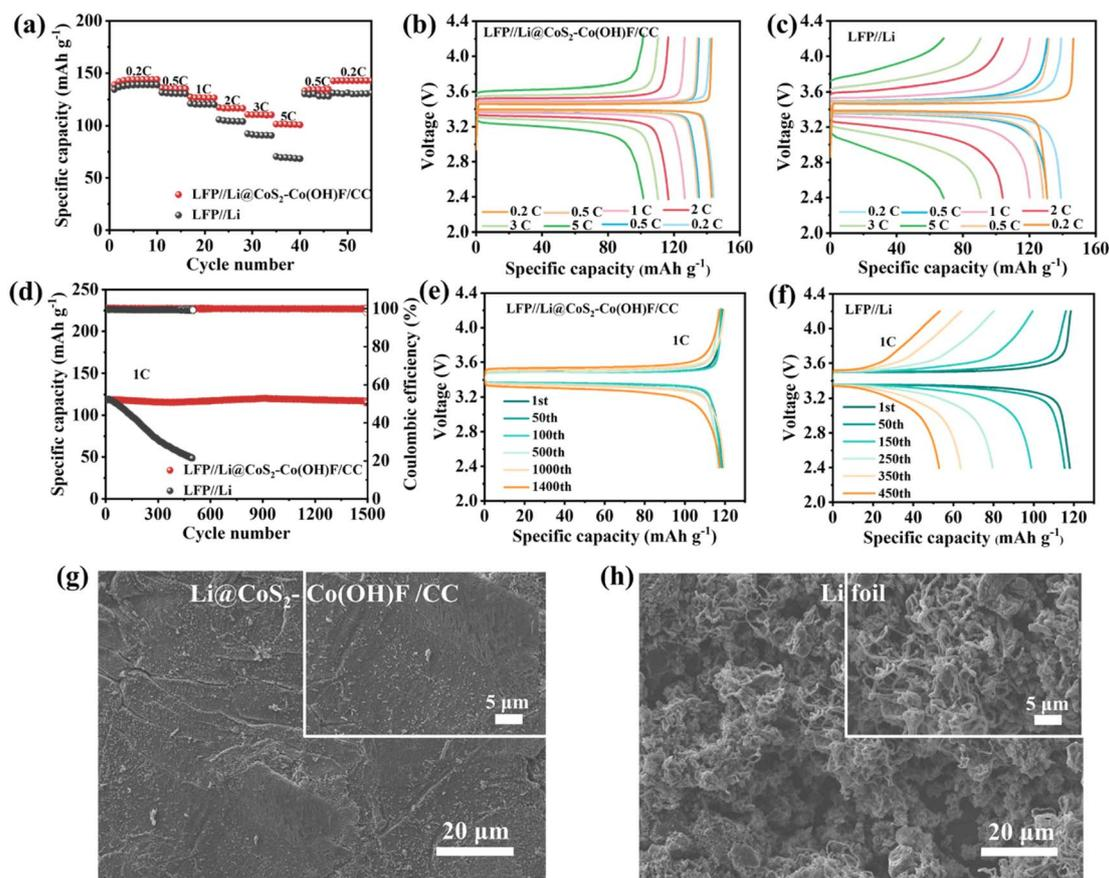
Fig. 7 (a) Rate capability and (b and c) charge–discharge profiles of LFP//Li@Li@CoS<sub>2</sub>–Co(OH)F/CC and LFP//Li full cells at various rates ranging from 0.2C to 5C. (d) Cycle performance and (e and f) charge–discharge profiles of LFP//Li@CoS<sub>2</sub>–Co(OH)F/CC and LFP//Li full cells at 1C. The SEM images of the corresponding anode for (g) LFP//Li@CoS<sub>2</sub>–Co(OH)F/CC and (h) LFP//Li full cells after 200 cycles at 1C.
