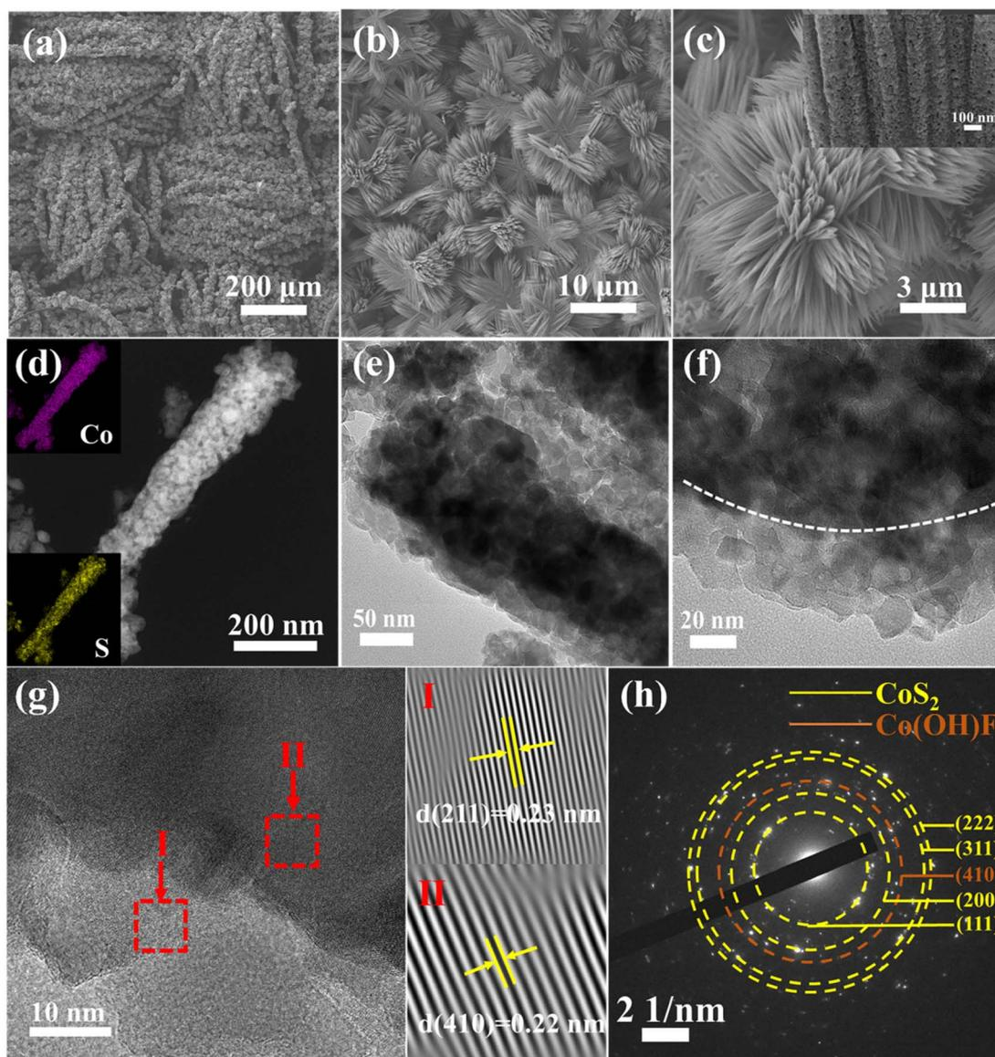
Fig. 2 (a–c) SEM images of  $\text{CoS}_2\text{-Co(OH)F/CC}$  nanowire clusters at different magnifications. (d) Elemental mapping, (e–g) TEM images, and (h) SAED pattern of the  $\text{CoS}_2\text{-Co(OH)F}$  nanorod.
