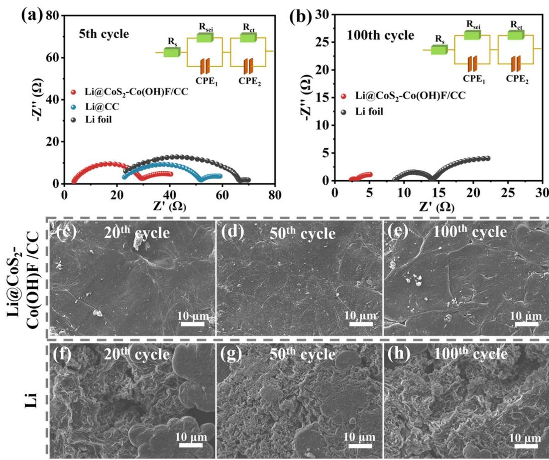
Fig. 6 (a and b) Nyquist plot of Li foil, Li@CC and Li@CoS<sub>2</sub>-Co(OH)F/CC-based symmetric cells at different cycles. SEM images of (c-e) the Li@CoS<sub>2</sub>-Co(OH)F/CC and (f-h) Li foil electrode after different cycles.
