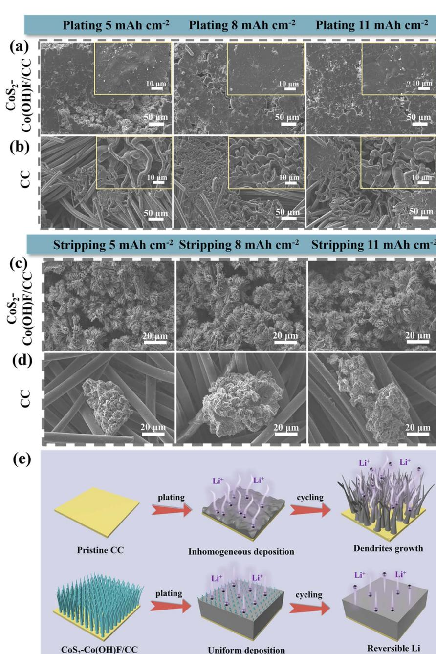
Fig. 4 SEM images of the (a) CoS<sub>2</sub>-Co(OH)F/CC framework and (b) CC after plating different amounts of Li. SEM images of the (c) CoS<sub>2</sub>-Co(OH)F/CC framework and (d) CC after Li stripping. (e) Schematic illustration showing the mechanism of the 3D CoS<sub>2</sub>-Co(OH)F/CC skeleton in suppressing Li dendrite growth.
